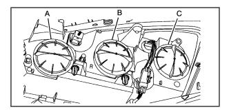
4. Remove the dust covers (A, B, or C) from the individual bulb sockets.
